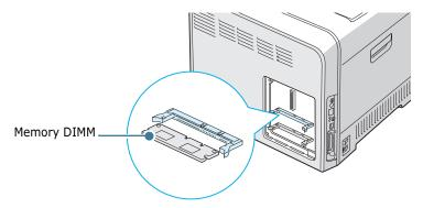
**5** Open the lever on each side of the memory DIMM slot all the way.
